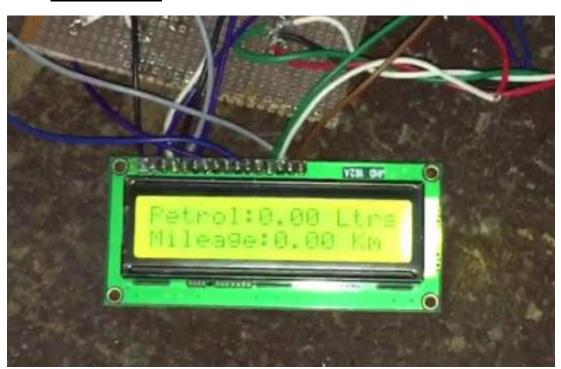
Digimetre is a digital fuel tank which will show how much petrol is there in tank (in Litres). All the values will be in digital format. It will also show how much petrol is poured in the tank at petrol pump in order to avoid frauds. It will also provide the mileage showing how much the vehicle can be driven in the remaining petrol
