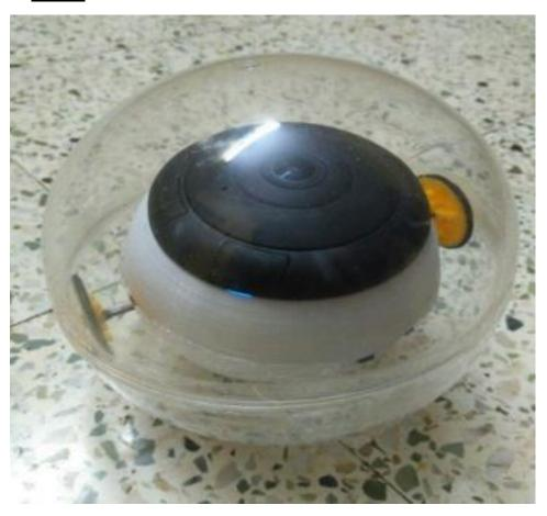
STAB is a Surveillance Transparent Arduino based Bot. This bot consists of a ball within another ball. The inner ball won't move at all, its only the outer ball that moves. The inner ball contains camera and circuits. The bot can move and can be controlled using controllers. These bots can be used for doing proper surveillance in areas before sending armies. The camera will send the live status on the screen which can be installed on any army group leader's glove.
