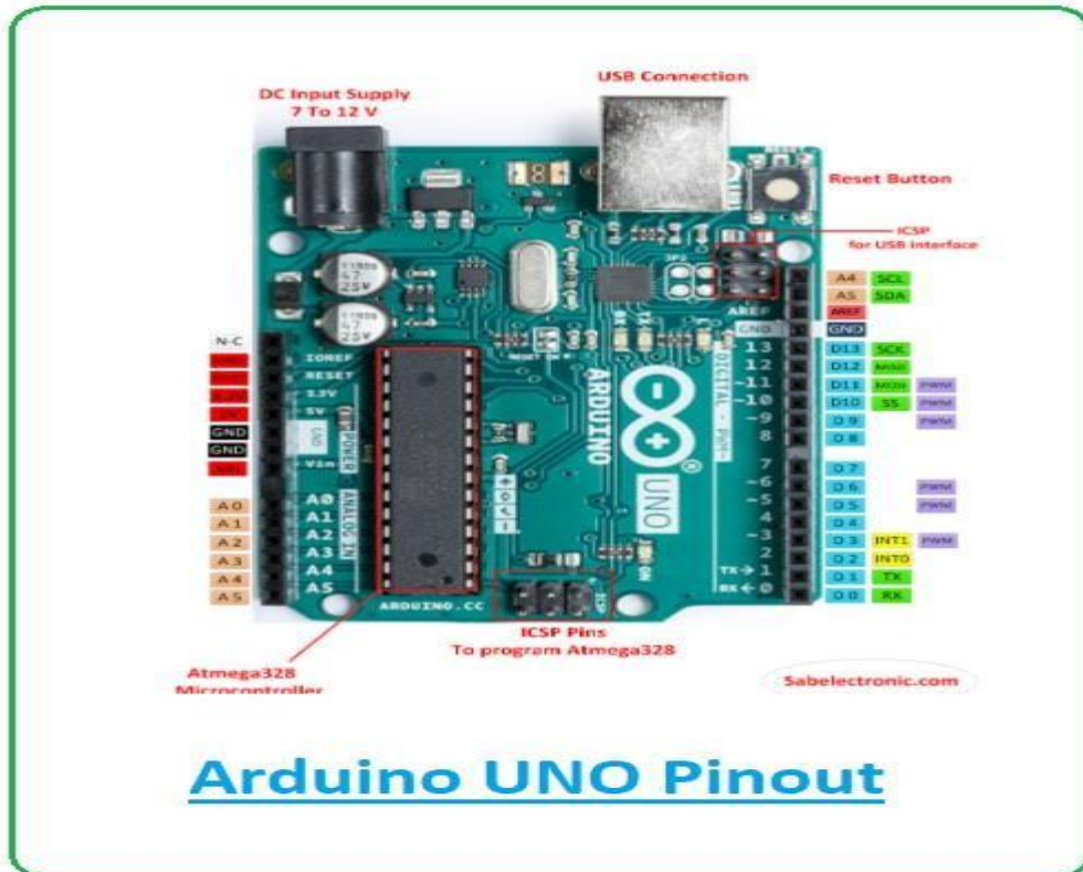
Figure 3.1.5 Arduino UNO Pinout
